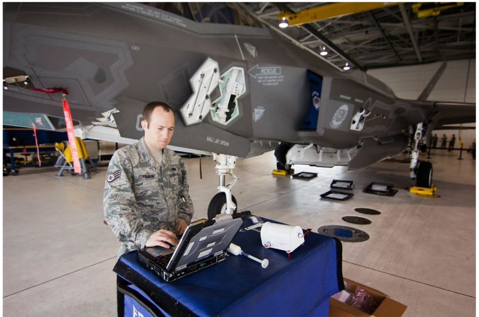
Figure 8: A Maintainer Using a Portable Maintenance Aid to Navigate ALIS Applications
