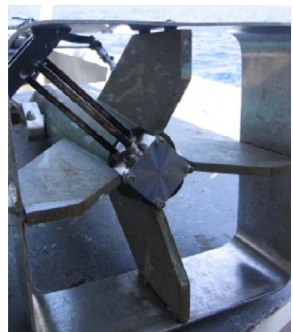
Figure 4. AML SV&P sensor (on single sensor fish)
